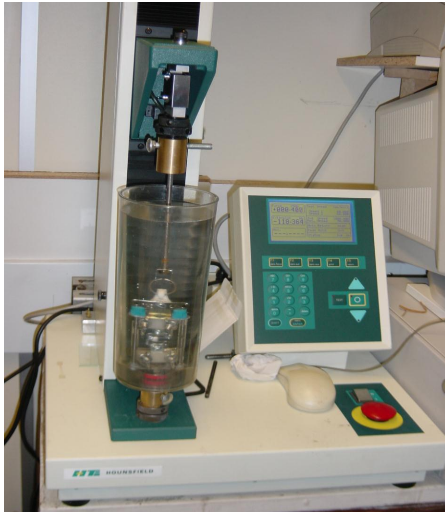
Fig 5.11. The tensile test including environmental chamber filled with water at 37°C.
