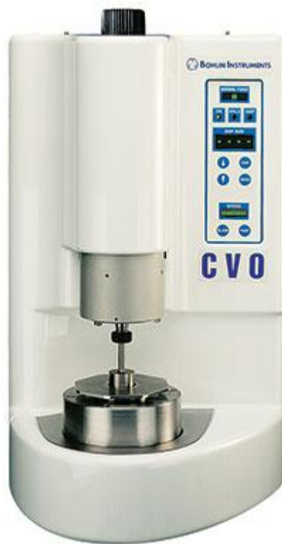
Fig 6.9. Bohlin CVO Rheometer – 4° cone and plate type, with full rheological testing capabilities including temperature adjustment using a Peltier plate system.
