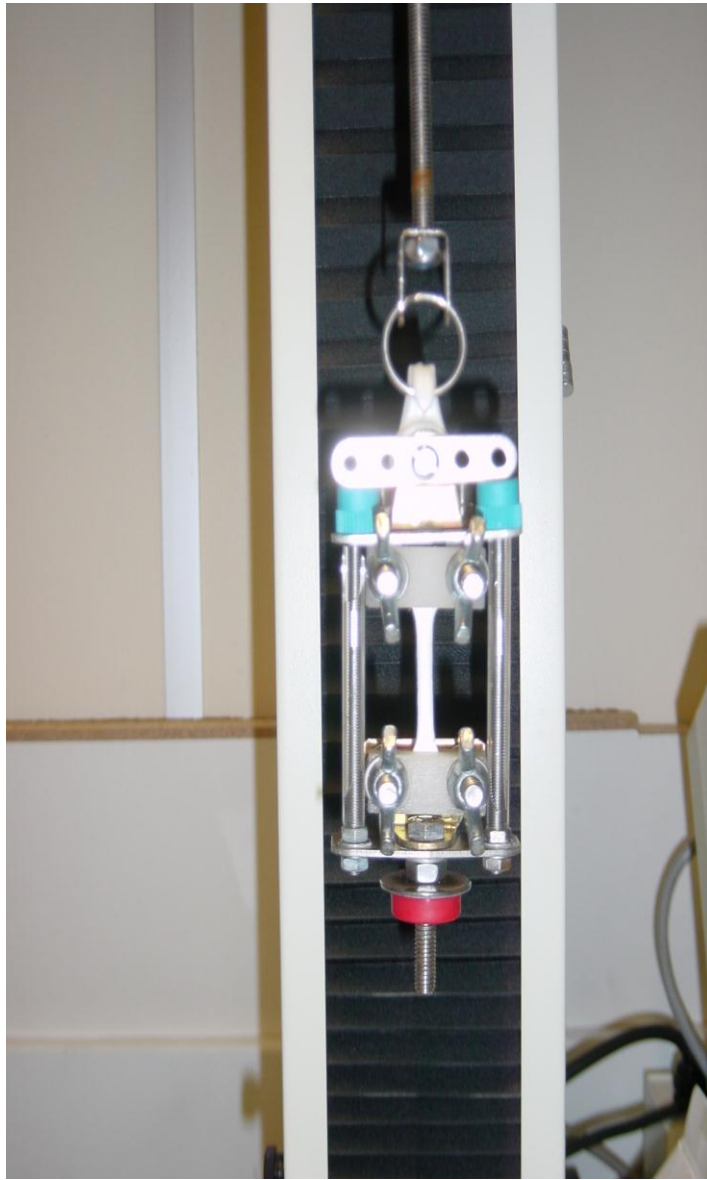
Fig 5.8a. The longitudinal sample held in the neutral position within the nylon block grips.
