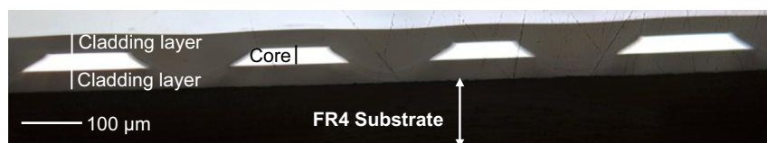
Fig. 4. Optical microscope images showing four adjacent waveguides machined using a CO 2 laser in Truemode™ acrylate photopolymer at an input power of 4.0 W and speed of 100 mm/s.
