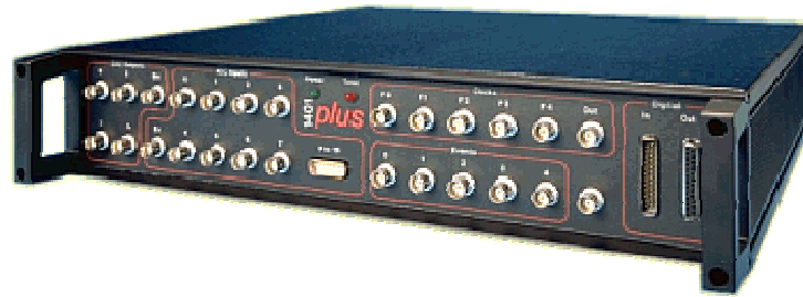
Figure 6:2 – CED 1401 plus data acquisition system, act as an interface to the real time analogue signal and SPIKE digital signal [176].
