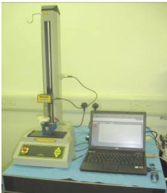
Figure 2.10 Showing the mechanical tensiometer device (Mecmesin) connected to a laptop. Force readings were measured and recorded using Emperor Software (supplied by Mecmesin).
