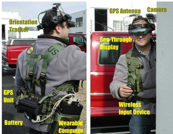
Figure 1. The problems of tracker alignment are exacerbated when multiple tracking systems are used simultaneously. This mobile system uses an inertial navigation system and a GPS.
