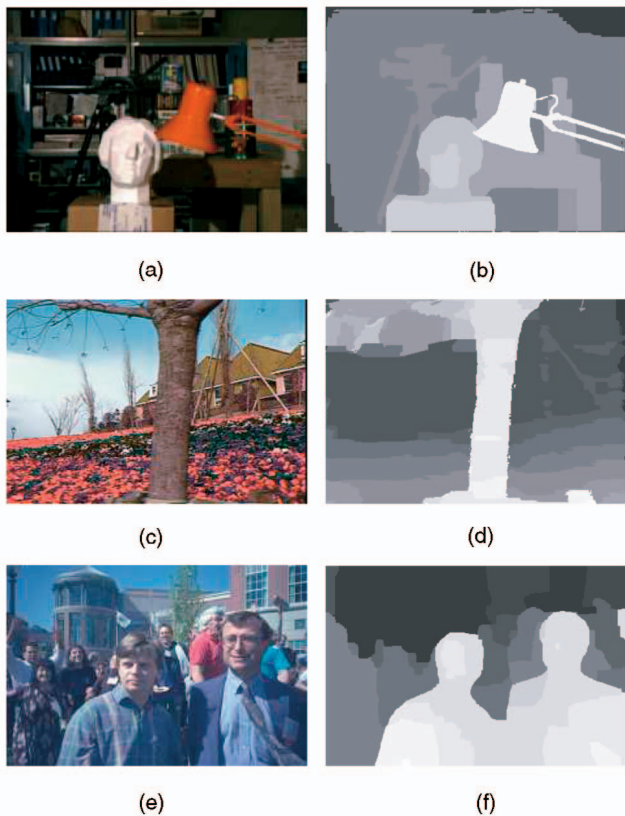
Fig. 10. Multicamera reconstruction results. There are five images of size 384 \times 288 in (a), eight images of size 352 \times 240 in (c), and five images of size 384 \times 256 in (e). (a) Middle image of Head data set. (b) Scene reconstruction for Head data set. (c) Middle image of Garden sequence. (d) Scene reconstruction for Garden sequence. (e) Middle image of Dayton sequence. (f) Scene reconstruction for Dayton sequence.
