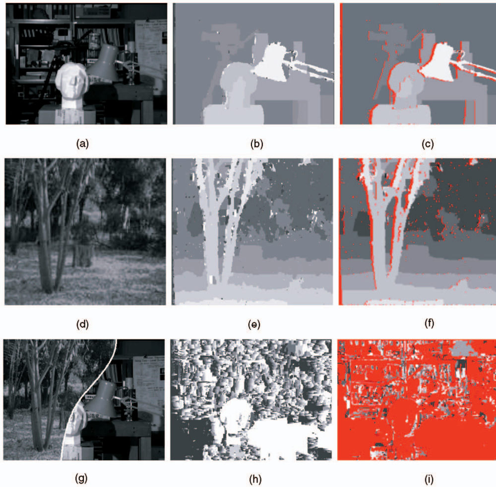
Fig. 9. (a) Left image of Head pair. (b) Potts model stereo. (c) Stereo with occlusions. Disparity maps obtained for the Head pair. (d) Left image of Tree pair. (e) Potts model stereo. (f) Stereo with occlusions. Disparity maps obtained for the Tree pair. (g) Random pair. (h) Potts model stereo. (i) Stereo with occlusions. Disparity maps obtained for the Random pair. Stereo results. The sizes of images are 384 \times 288 in (a), (b), and (c). 256 \times 233 in (d), (e), and (f). 384 \times 288 in (g), (h), and (i). The results in (c), (f), and (i) show occluded pixels in red.
