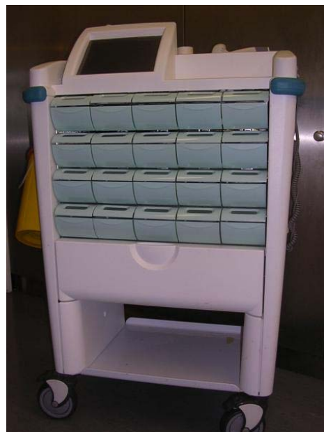
Figure 4: One of the two electronic drug trolleys. One drawer is allocated to each patient for whom medication is due and their name shown on the liquid crystal display. The barcode scanner is on the top of the trolley.
