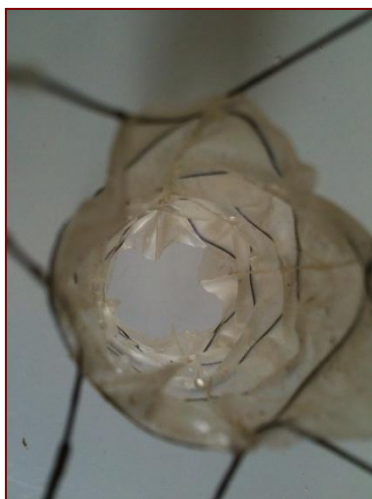
Figure 5.5: Images of the stent-grafts post-fatigue testing. Visual inspection revealed intact polymer and nitinol with no signs of breakage.
