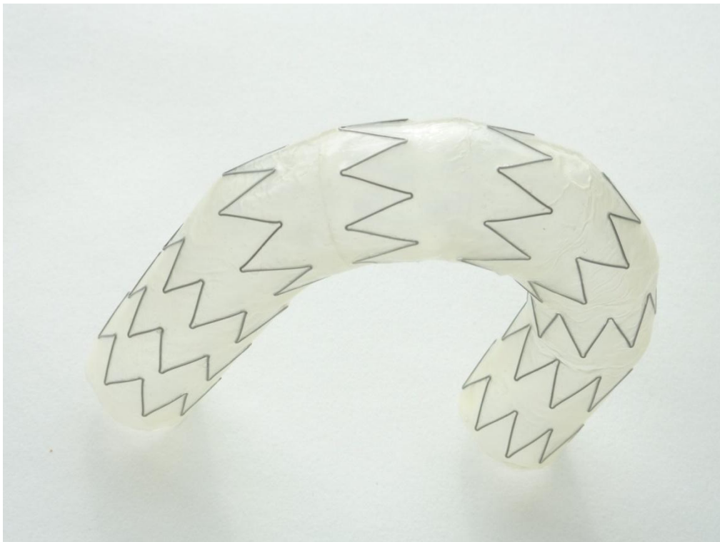
Figure 3.14: A curved stent-graft in fully expanded shape and matching curvature of aortic arch
