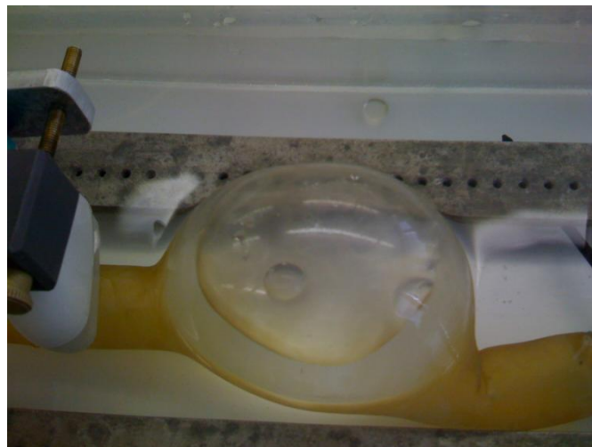
Figure 4.5: Latex model showing significant distension on increasing mean pressure from 90 mm Hg to 120 mm Hg
