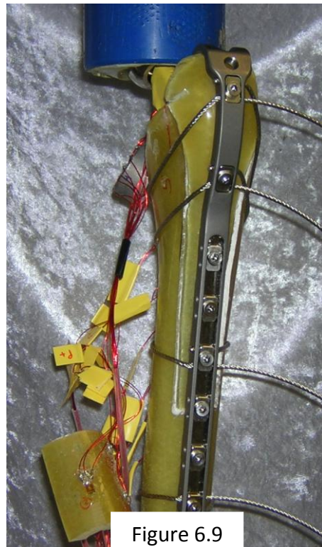
Figures 6.6 – 6.9: Composite femur models fixed with 2 cables and a strut(6.6), 3 cables and a strut (6.7), short trochanteric grip (6.8) and long trochanteric grip (6.9)
