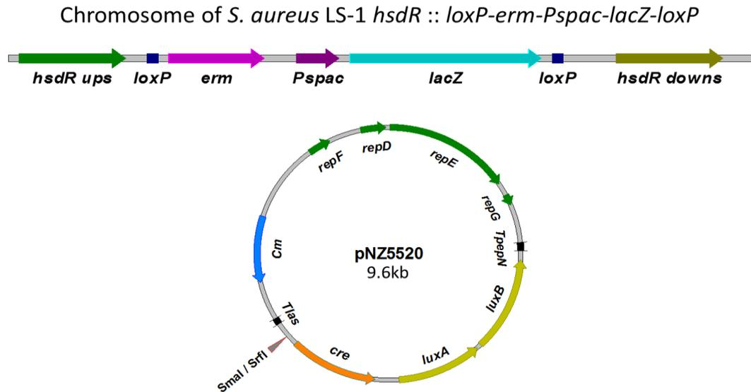
Figure 4.10: Schematic diagram of the *S. aureus* R-IVET system (not drawn to scale). The *loxP-erm-Pspac-loxP* cassette is integrated into the chromosome of *S. aureus* LS-1 between loci SAOUHSC\_00161 and SAOUHSC\_00163 according to the locus tags in *S. aureus* NCTC 8325. The plasmid pNZ5520 contains the reporter genes *cre*, *luxA* and *luxB*, and a *SfrI*/*Smal* restriction site upstream of *cre* is for the insertion of chromosomal fragments.
