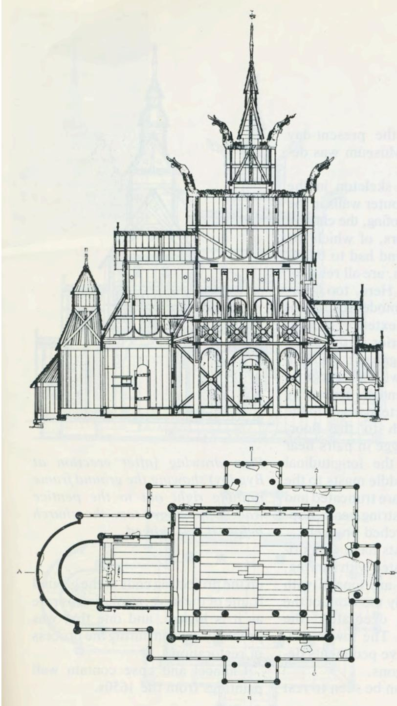
Figure 7: Borgund stave church: plan and long section. (Bugge G. *Stave-churches in Norway*. Dreyers Forlag A/S (1983) p65.)
