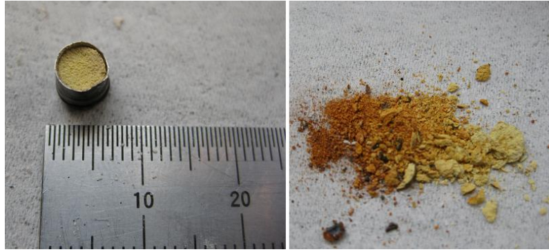
Figure 15. Extracting the sample from the capsule after a piston cylinder experiment.
