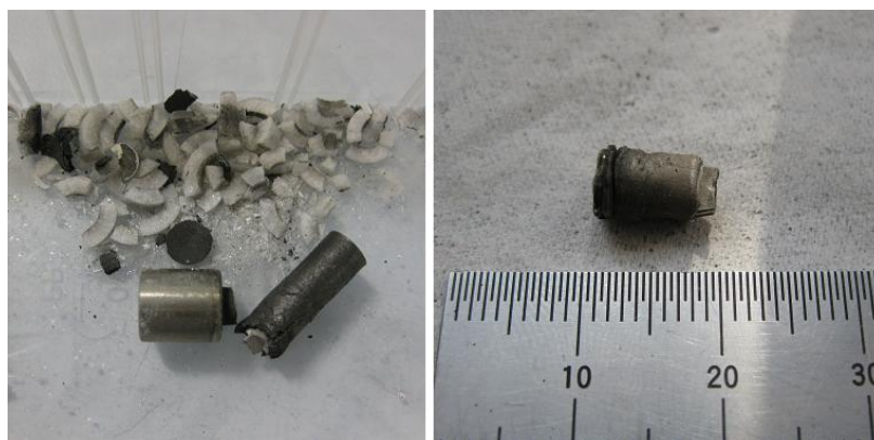
Figure 14. Removing the sample capsule from the piston cylinder assembly after compression.
