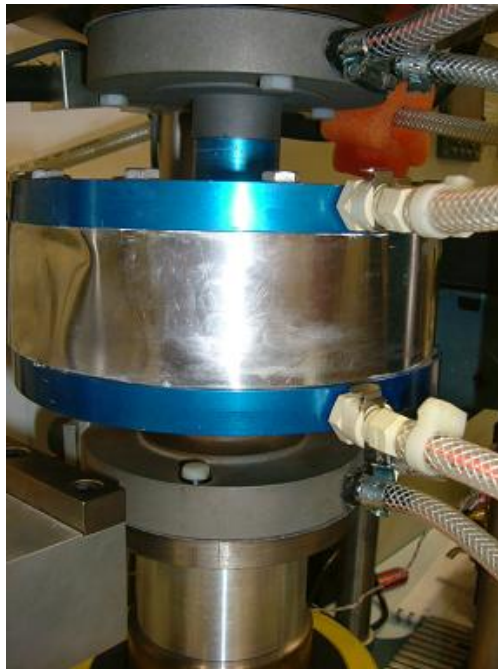
Figure 11. Schematic Diagram of Run Position (top). Pressure plate in run position (bottom) in the piston cylinder apparatus.
