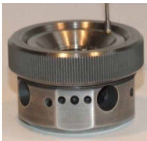
Figure 23. The Diacell ® Bragg (G) type diamond anvil cell used for some of this work.
