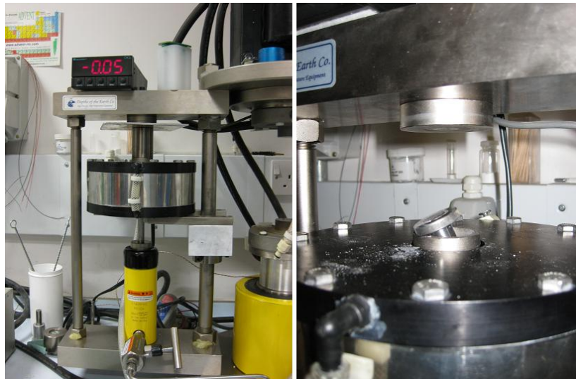
Figure 13. Extraction of the sample assembly from piston cylinder.
