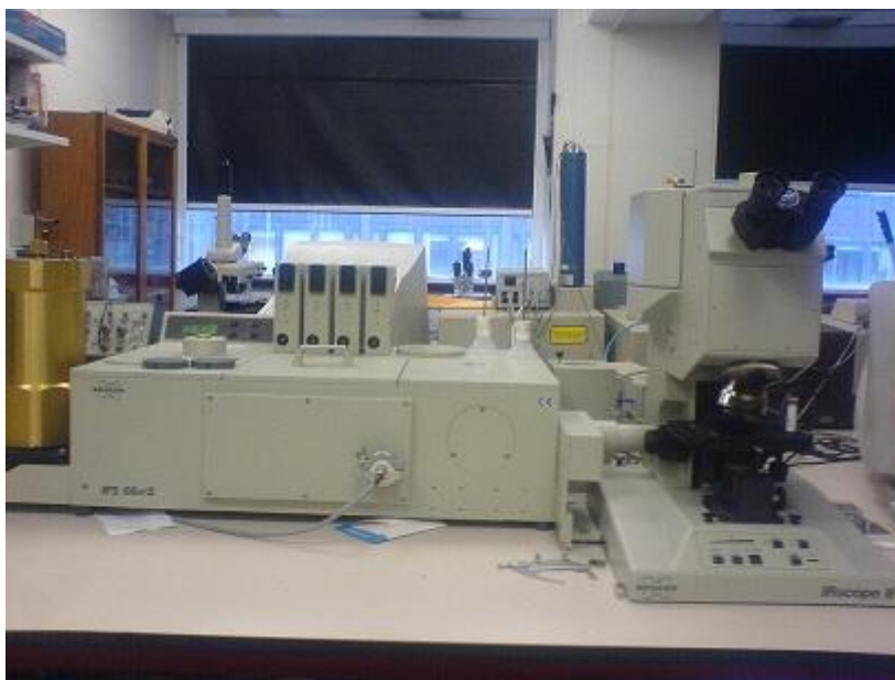
Figure 38. The Bruker IFS 66v/S FTIR spectrometer with IRscope II infrared microscope used to take the IR spectra.
