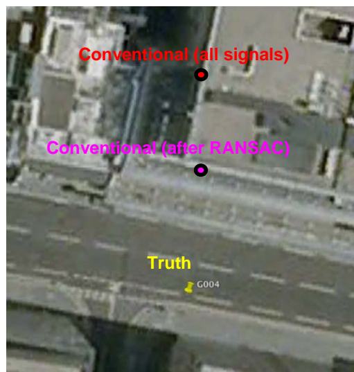
Figure 8: Conventional GNSS position solutions before and after application of RANSAC-based consistency checking
