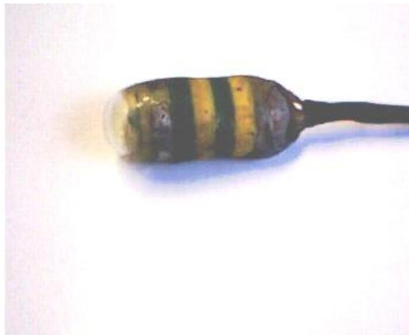
Fig. 4.22 Video endoscope capsule with attached electrodes.
