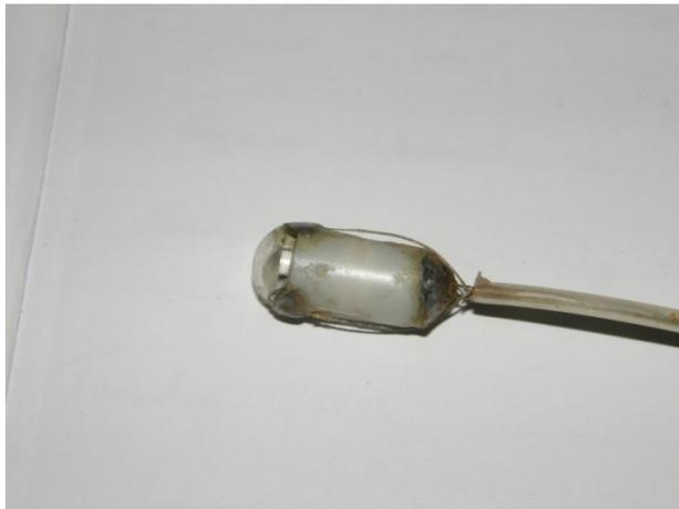
Fig. 4.20 Bidirectional video capsule endoscope
