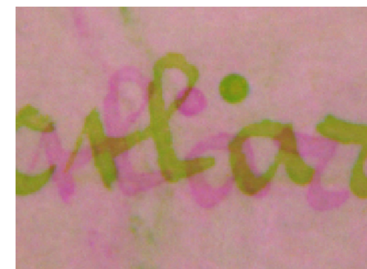
False-colour composite of reference 600 nm channel of sample before treatment (blue), 850 nm channel of sample after treatment (green), and the latter after registration (red).
