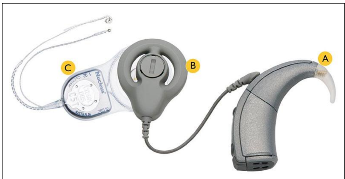
Figure 1.3 Picture of the CI device; (A) external behind the ear speech processor; (B) the transmitting coil and (C) the internal implant with the receiver, stimulator and electrode array; courtesy of Cochlear®
