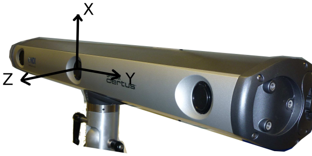
Fig. 2. The coordinate system of the Optotrak Certus. The z axis is aligned with the surface normal of the central camera.
