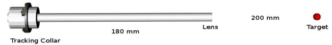
Fig. 15. The geometry of the laparoscope tracking model. The laparoscope modelled has a distance of 180 mm from the tracking collar to the lens. The surgical target is a further 200 mm in front of the laparoscope lens. Though the pose of the laparoscope changes during the simulation to achieve different IRED normal angles, the position of the target remains fixed with respect to the laparoscope lens, i.e. the target moves relative to the coordinates of the tracking camera system or “operating room”.
