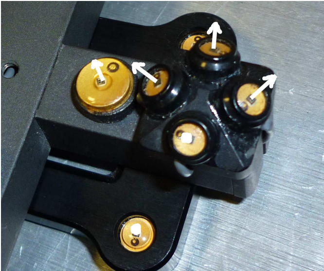
Fig. 5. An example of surface normal vectors on the cross rigid body
