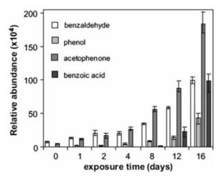
Figure 6 Relative abundance of detected low-molecular weight compounds from samples of HIPS following different periods of thermo-oxidative degradation. Reprinted from Vilaplana *et al.* (2010) with permission from Elsevier.
