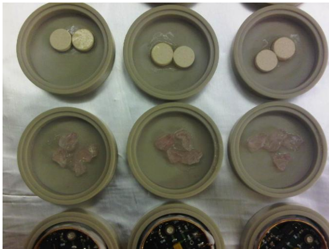
Figure 6.10 Molecular sieve (top) and silica gel (bottom) desiccant in PEEK capsules
