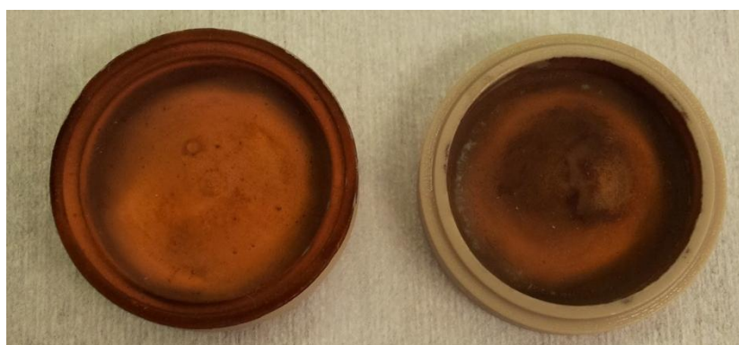
Figure 7.38 PEEK capsule electroplated with copper
