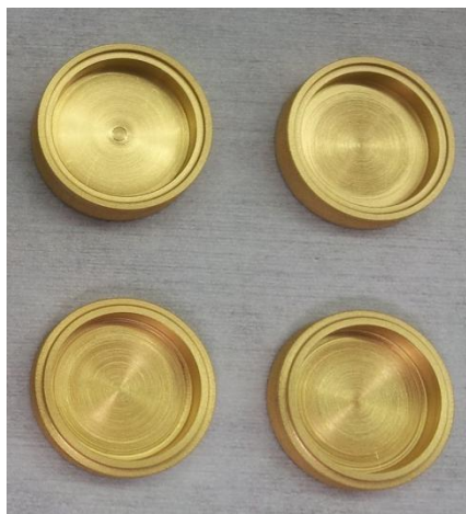
Figure 7.29 Ar sputtering of PEEK capsules with (from left to right): Ti+Au and Cr+Au (500 nm thickness)
