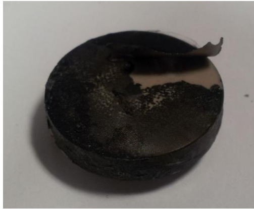
Figure 7.34 DLC coating peeling off
