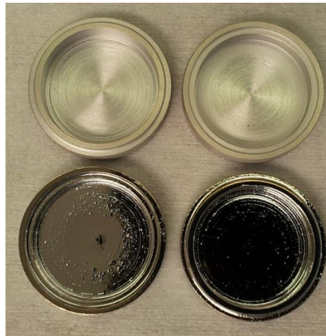
Figure 7.19 PEEK capsules with evaporation deposited aluminium thin film - with (bottom) and without (top) base lacquer applied beforehand and stoved
