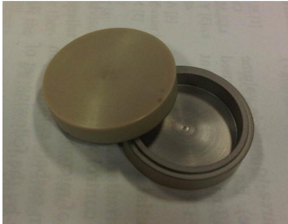
Figure 7.6 PEEK Capsule with 3 m Ti coating (CAD)
