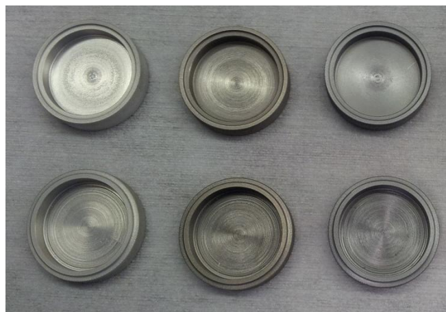
Figure 7.26 Ar sputtering of PEEK capsules with (from left to right): Al, Ti, and Cr (500nm thickness)
