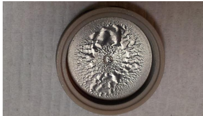
Figure 7.25 Zr coated PEEK capsule (magnetron sputtering) - blistering of the film
