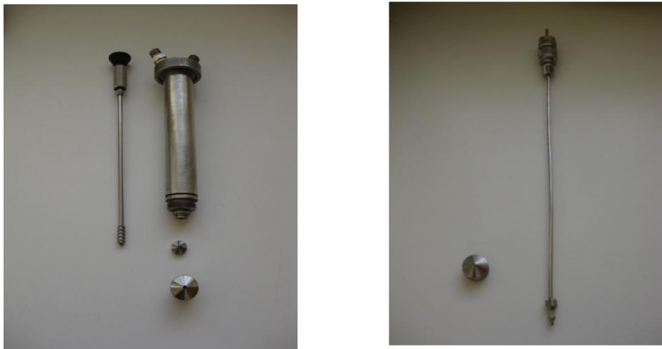
Figure 4-19: Büchi Spray Dryer Nozzle compared to the Niro Spray Dryer Nozzle Used
