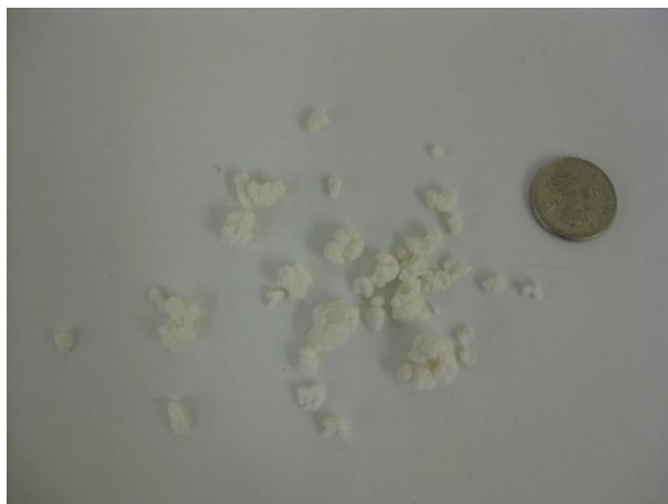
Figure 4-29: The large size of F1 Particles Produced at Solids Concentration 20 % w/v when compared to a coin
