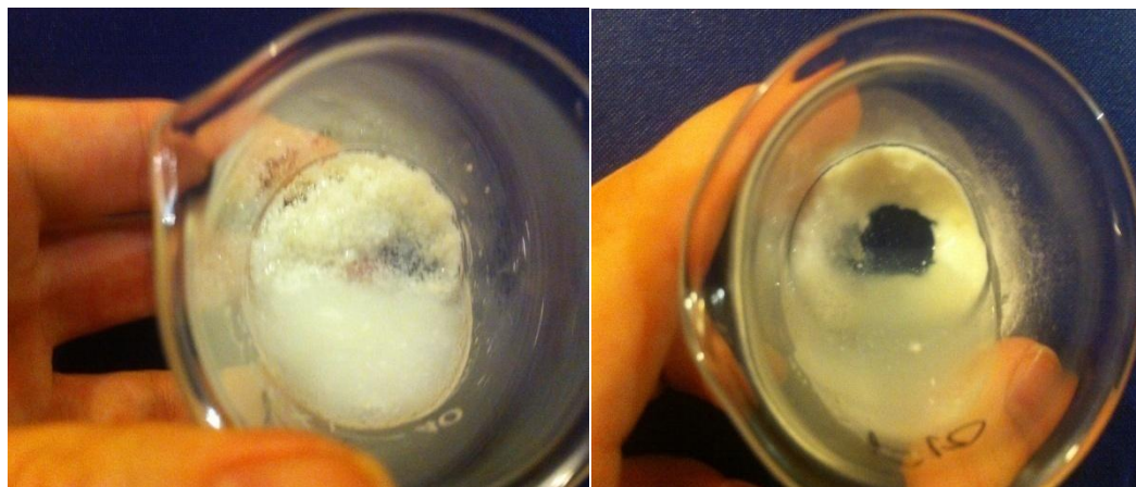
Figure 4-38: An assessment of the Suspendability of Larger Particles (<1 mm) of F9 (left) and Smaller Particles (>25 \mu\text{m} ) of F18 (right) at 1g of particles/40 ml of media. It can be seen that the larger particles are difficult to suspend and sediment to the bottom whereas the lighter particles appear to be compacted by the addition of the media and sticks to the bottom/sides of the beaker
