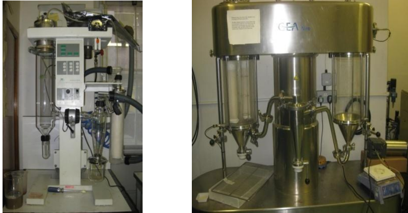
Figure 4-17: Büchi Spray Dryer (Left) compared to the Niro Spray Dryer Used (Right)
