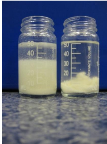
Figure 2-20: Dispersion of Cellets® (200 µm) after stirring in a Beaker in MC 1 % (left) and 3 % (right)
