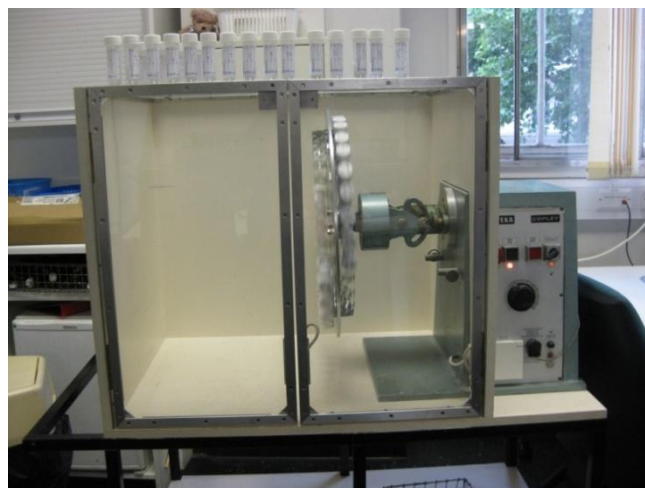
Figure 2-23: Mechanical Wheel used to try to Keep Particles Suspended in Samples for Grittiness Trials (after the particles had been dispersed by stirring/mixing/shaking until just prior to administration)
