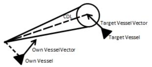
Figure 1. Construction of a collision danger sector (CDS).
