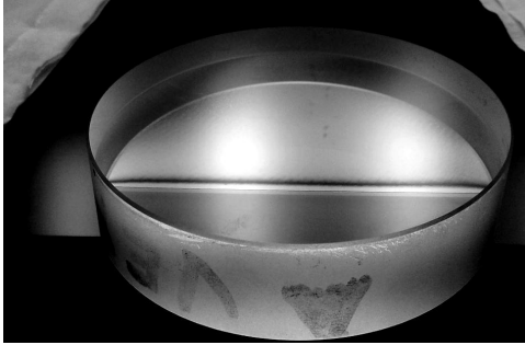
Figure 11a Test plate result showing induced edge up-stand
