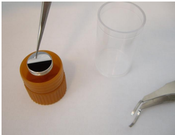
(Clockwise from top-left): Figure 4.7 Sample stubs in labelled sample tubes, pre-sampling
