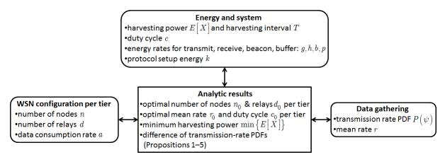
Figure 4. Conceptual illustration of the linkage between: network, system and data gathering via the proposed analysis. When parameters from two out of three domains are provided, our analytic framework can tune the parameters of the third. The symbol definitions are provided in Table I.
