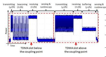
Figure 2. Energy profile of a TelosB sensor node within an undercoupled and an overcoupled TDMA slot during the active period. The indicated metrics (in Joule-per-bit) are defined in Table I.
