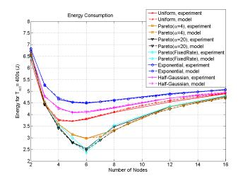
Figure 5. Energy consumption per node under different data transmission PDFs. The experiments correspond to  $T_{\rm act}$  = 400 s, k = 165.6 mJ and d = 0.
