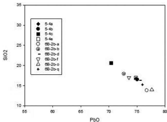
Figure 9: Silica (SiO<sub>2</sub>) and lead oxide (PbO) content of the slag samples from Banc Tynddol (XRF analyses).
