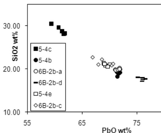
Figure 10: Silica (SiO<sub>2</sub>) and lead oxide (PbO) content of the glassy matrix of the slag samples from Banc Tynddol (SEM-EDX analyses).
