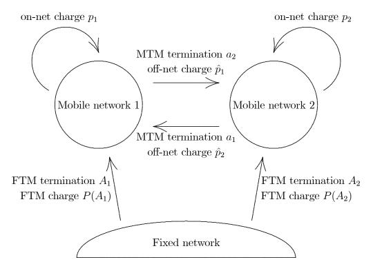
Fig. 1: Call Termination on Mobile Networks
