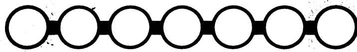
Figure 1.3: Permanently coupled quantum chains can transfer quantum states without control along the line. Note that the ends still need to be controllable to initialise and read out quantum states.
