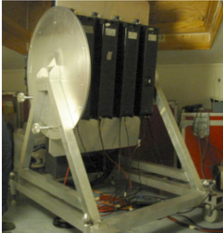
Figure 2.8 The SIF platform in its dome in Svalbard, showing the four photometers. The spectrograph and TLC are on the other side of the back plate.
