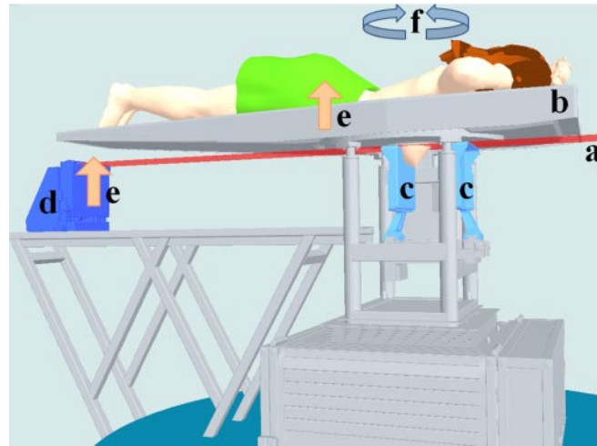
Fig. 16. – Sketch of the imaging system for phase contrast mammography with synchrotron radiation: (a) stationary and laminar X-ray beam, (b) movable patient support, (c) compression system, (d) holder for screen-film cassette, (e) vertical scanning movement of the patient and of the screen-film system through the beam, which allows the acquisition of planar radiographic images, (f) rotational movement of the patient, which allows both the craniocaudal and mediolateral oblique views to be obtained. Reproduced, with permission, from Castelli et al. Radiology , 259 (2011) 684 (supplementary material).
