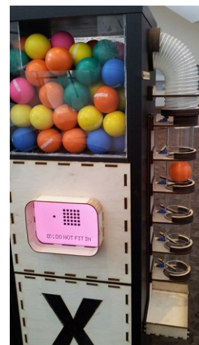
Figure 6. The ball tube at the side of the system functioned as an incentive for completion and progress indicator.
