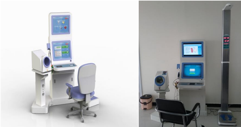
Figure 11: The finalized design and the implementation of the healthcare kiosk.
