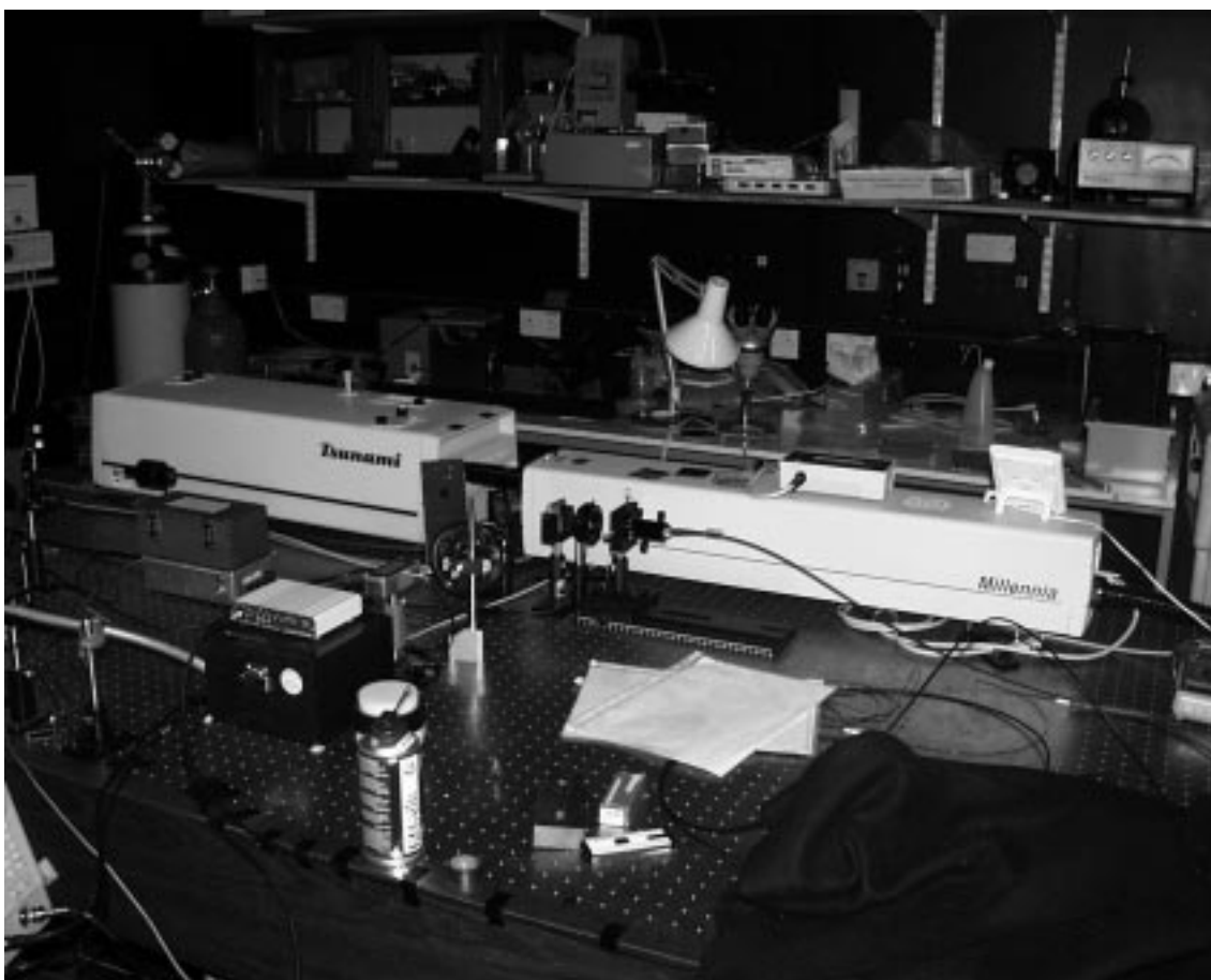
Figure 6.40 Photograph showing the laser table in our laboratory. The right hand laser is the Millennia pump laser producing 5 W at 532 nm. The laser to the left is the infra-red Tsunami laser, tunable from 720 to 840 nm.
