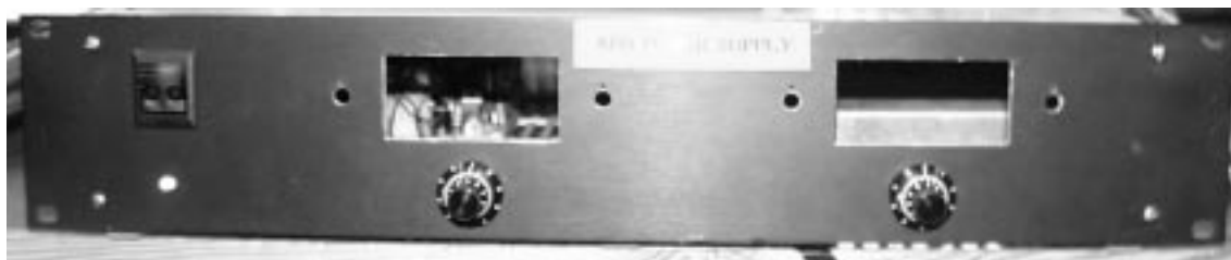
Figure 6.39 Photograph showing the APD power supply. The holes in the front panel are for two digital voltage meters, which were never fitted.
