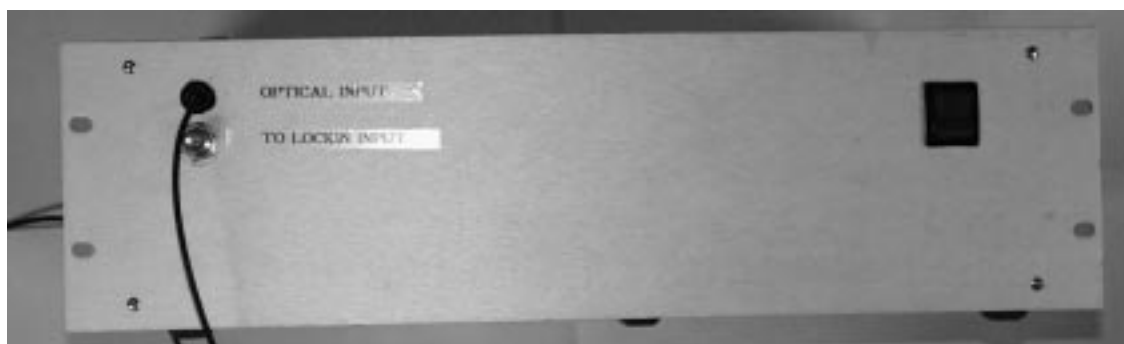
Figure 6.36 Front view of the main electronic enclosure for the cross-correlator. The detection fibre can be seen to the left. The BNC socket shown connects to the lock-in amplifier input.
