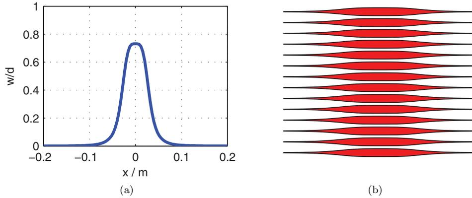
FIG. 9. (a) The ratio between the width of the strip  $w$  and the side length of the unit cell  $d$  as a function of  $x$  throughout the resonator. (b) Schematic drawing of the resonator near  $x = 0$ .
