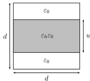
FIG. 8. The structure of one MM cell in the lattice that forms the effectively homogeneous 2D SRO material. Each cell consists of a horizontal strip of material with a high permittivity  $\epsilon_h\epsilon_0$ , embedded in the background material with permittivity  $\epsilon_0$ . These cells are assembled horizontally with varying fill ratios  $w(x)/d$ , and the resulting strips then stacked vertically.
