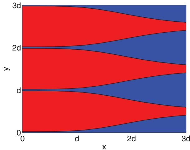
FIG. 3. *SRO metamaterial. Schematic top view of a 2D SRO medium for electromagnetism at subwavelength scale  $d$  near the axis  $x = 0$ . MM cells are grouped to form  $x$ -directed strips of varying width  $w(x)$  and high permittivity (red), embedded in background material with relative permittivity  $\varepsilon_r = 1$  (blue). The inhomogeneity in  $x$  of the strip widths is crucial for the various superdimensional properties of the material. Color is available online only.*
