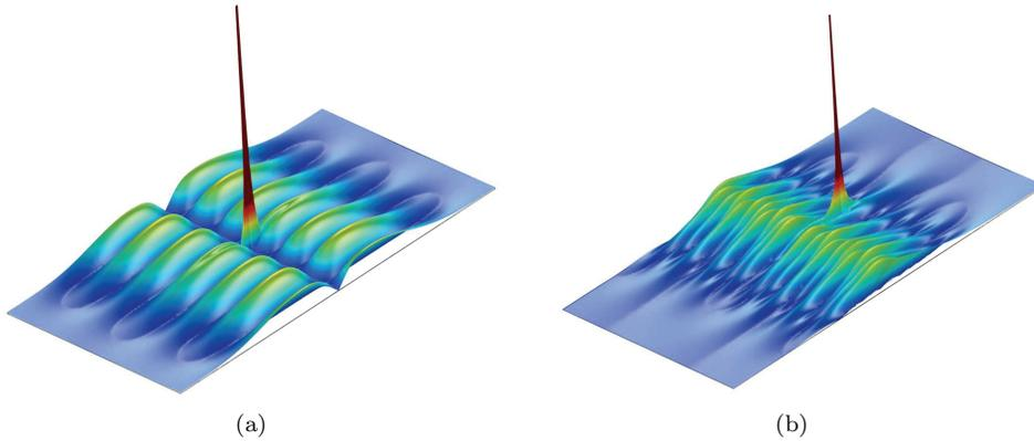
FIG. 11. (a) Superdimensional electromagnetic resonator with material parameters (27) excited by a  $\mathbf{u}_y$ -polarized line dipole at  $(x', y') = (0, 0)$  at  $f = 1\text{GHz}$ . (b) Same as in (a) but with the dipole located at  $(x', y') = (0.05\text{m}, 0\text{m})$ .
