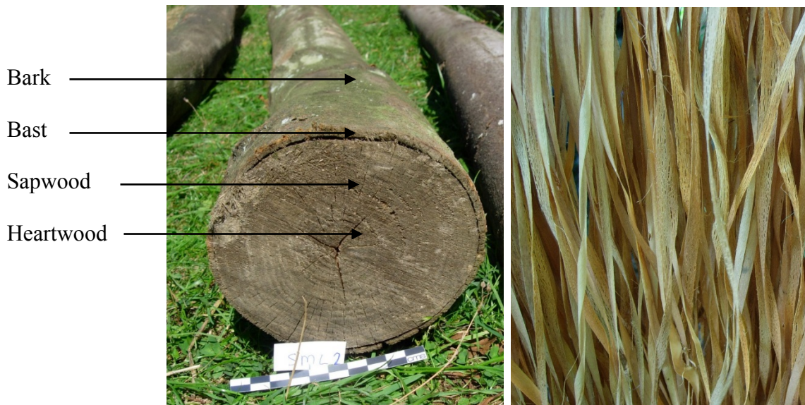
Figure 2. Left: Location of tree bast fibres in cross-section (image © Susanna Harris). Figure 3. Right: Processed lime bast fibres (image © Susanna Harris).
