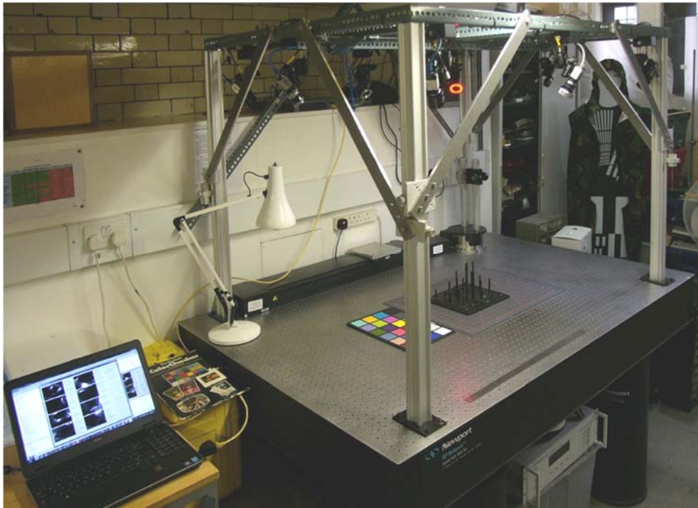
Figure 2. View of 8-camera test rig in laboratory.
