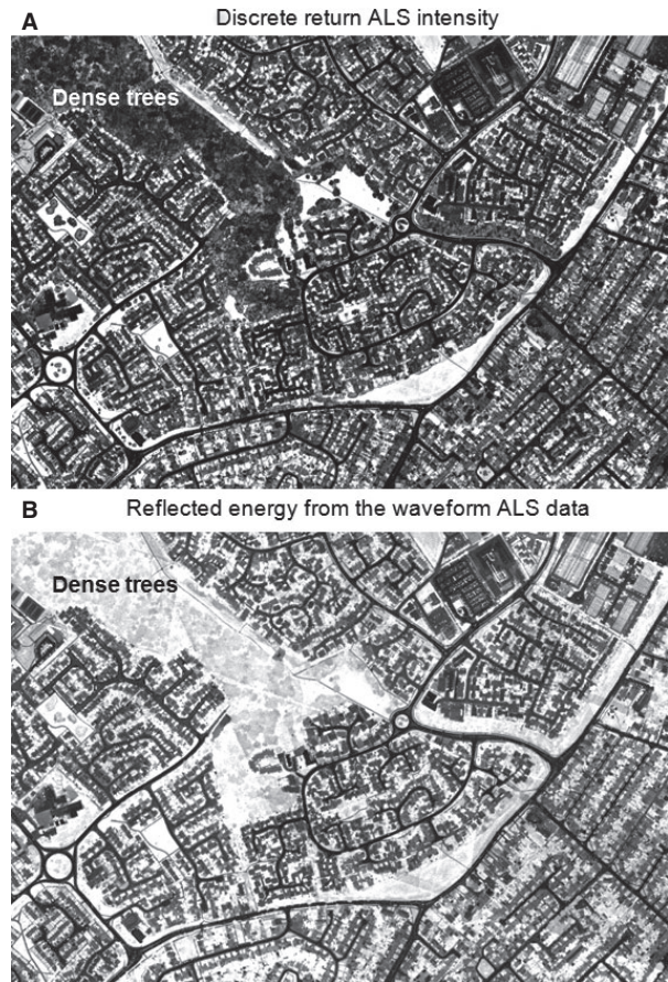
Figure 4. The impact of using discrete return intensity versus waveform airborne laser scanning (ALS) in the near infrared (1064 nm) is shown for a mixed zone in the focal area of Luton. In (A) the intensity of the discrete return ALS data are shown, while (B) shows the difference when waveform ALS intensity is used. The major differences in intensity appear in zones with dense vegetation. These data show that relying on discrete return intensity would lead to bias – the area of dense trees appear as having low intensity (low reflectance at 1064 nm) when they should have high reflectance (the two are related). This bias is not present in waveform intensity, which shows both the mown grass and the dense trees as having high intensity which is correct given the known strong vegetation reflectance response in this region of the spectrum.
