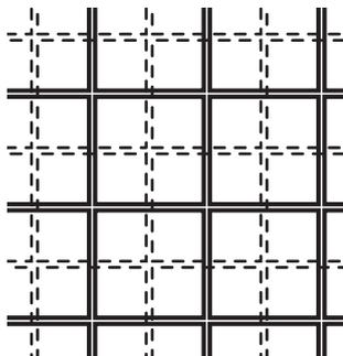
Figure 3.1: A schematization of the so-called Margolus partitioning scheme in  $s = 2$  dimensions. Operations are alternately applied to the solid and to the dashed partitioning into  $2 \times 2$  squares. Here cells are represented as squared, but their actual shape can be different, as it only serves to label localized quantum systems.
