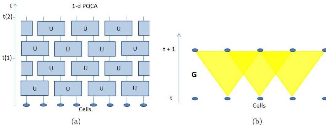
Figure 3.2: (a) Sketch of the 1-dimensional  $\frac{1}{2}$ -nearest neighbor QCA evolution in time. Wires are cells, time flows upwards. One iteration of the automaton corresponds to the application of two layers of local two-qubit unitaries. (b) The light cone of a QCA.
