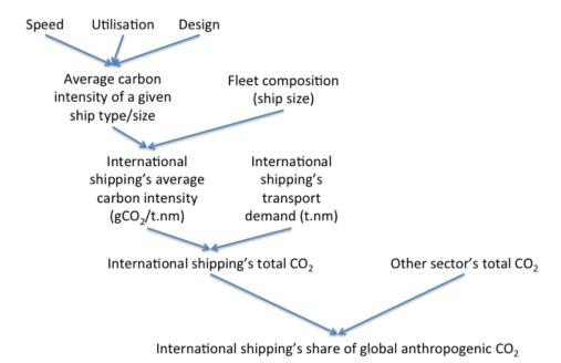
Figure 2, Diagram showing the interactions which contribute to shipping's CO<sub>2</sub> as a share of global anthropogenic CO<sub>2</sub>
