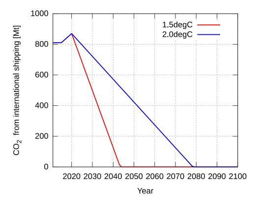
Figure 1, CO<sub>2</sub> emissions trajectories for international shipping consistent with a 2°C temperature rise (blue curve) and a 1.5°C temperature rise (red curve). The trajectories assume emissions as in the reference scenario from the Third IMO GHG Study 2014 to 2020, followed by constant reductions, with the year-on-year reduction determined by the remaining CO<sub>2</sub> emissions budget of 33Gt and 18Gt, respectively.
