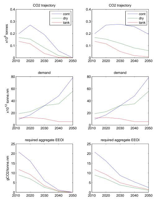
Figure 3: Estimation of trends in CO<sub>2</sub> trajectory and associated target operational CO<sub>2</sub> intensity trajectory consistent with 1.5°C (left hand side) and 2°C (right hand side)
