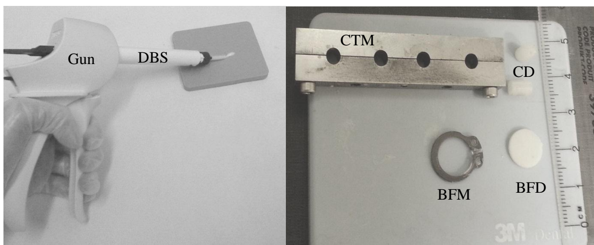
Figure 2.2 (a) Paste is extruded via mixing tip (b) Biaxial and compressive disc with their moulds. BFM; biaxial flexural mould, CTM; compressive test mould.
