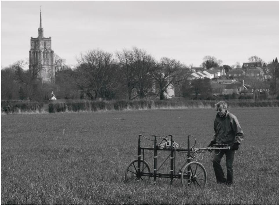
Figure 1: Jim West uses the Foerster Ferex magnetometer at Great Buttway, Ashwell End, Hertfordshire.
