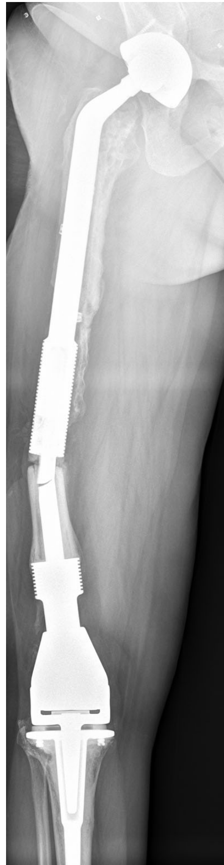
Figure 5: Full length femur radiograph illustrating fatigue fracture in stem of original distal femoral component.
