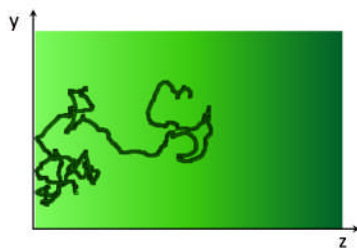
Figure 6 – Microalgal path according to the Langevin scheme of random walk in 3 mm bubble flow.
