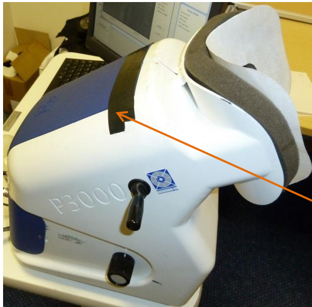
Slots for insertion of the NDF covered with tape
