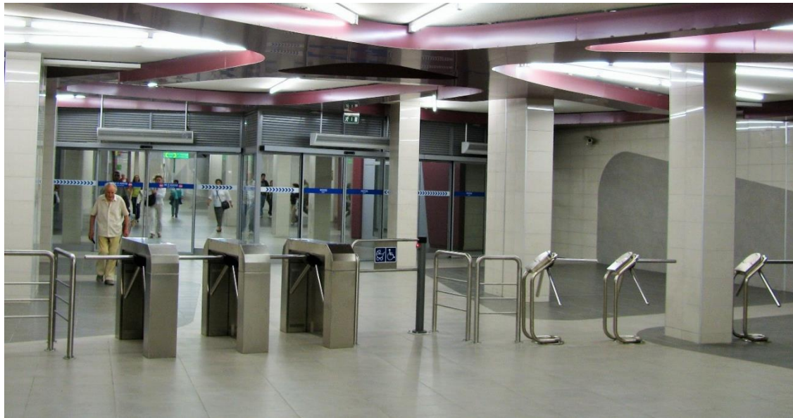
Figure 6-7: Different types of ticket barriers in the Sofia Metro. The second photograph shows the entry (left) and exit turnstiles in their typical position next to each other. September 2012. Photos by author.
