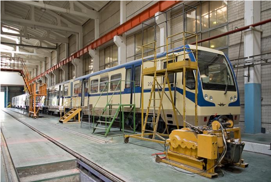
Figure 2-10. Train for the Sofia metro being assembled at MetroVagonMash plant. Source: Metroblog.ru
