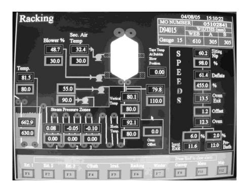
Figure 1. Screen shot of a part of the extrusion computer control system. White "thread" shows the
