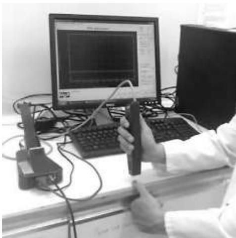
**Fig. 3.2** Photographic image of the TOWL instrument (Aquaflux) used to conduct film occlusivity tests.
