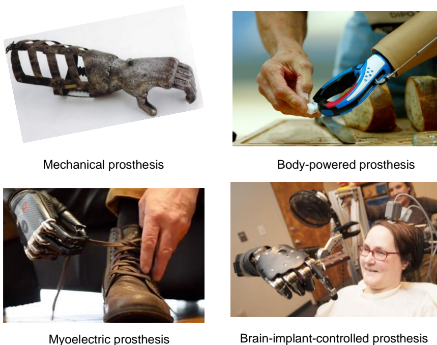
Figure 1 | Artificial arms for restoring hand function. a , An early mechanical prosthesis (ca. 1580) with movable joints for changing the static hand pose. b , A prosthetic arm that uses motions of the contralateral arm to operate the motion of the hook-like gripper. c , A bionic prosthetic arm that uses the readout of surface electromyography of the residual muscle to control pre-defined hand motions. d , Control of a multi-degree-of-freedom robotic arm by means of microelectrode array implants in the neocortex. Images courtesy of a , Peter Finer; b , TRS Inc.; c , Bebionic; d , University of Pittsburgh Medical Center.
