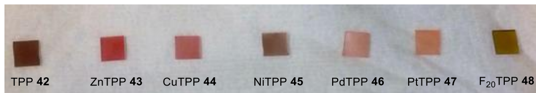
Figure 40. Silicone films that had been exposed to different porphyrin solutions for three days.
