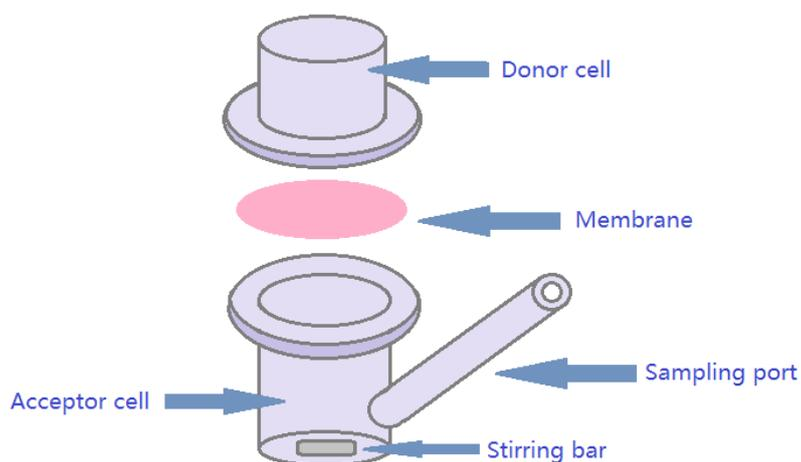
**Figure 3.1** Design of a typical Franz diffusion cell
