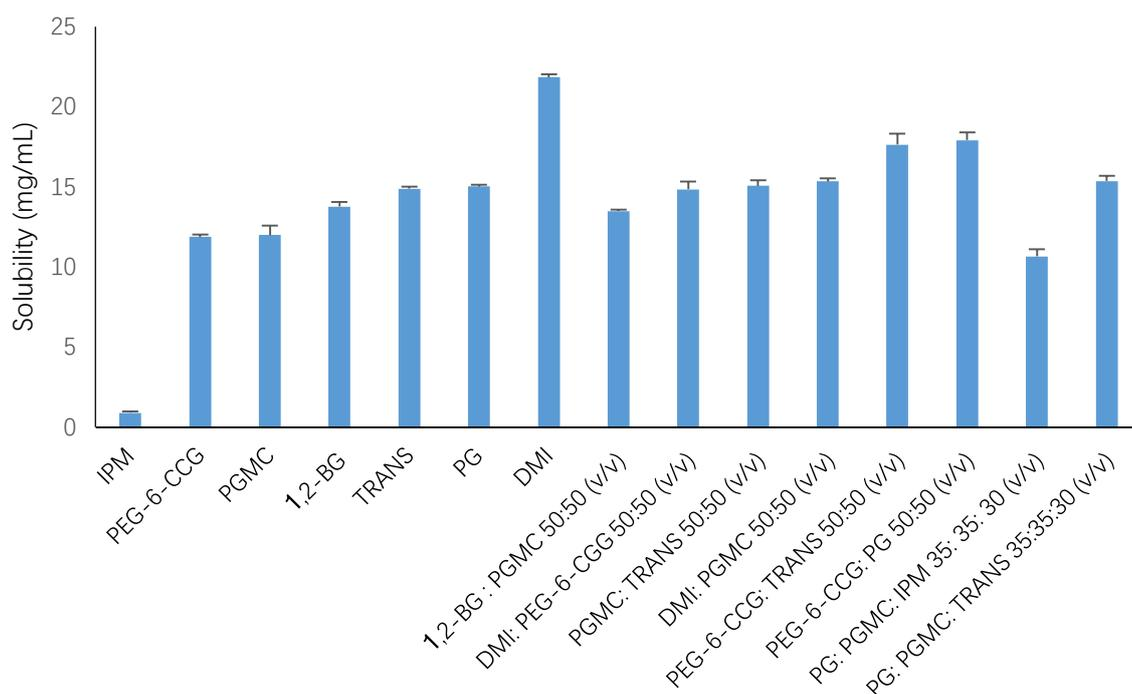
**Figure 6.12** Solubility of caffeine in a range of different solvents and solvent systems at  $32 \pm 1^\circ\text{C}$ . Each data point represents the mean  $\pm$  SD,  $n=5$ .
