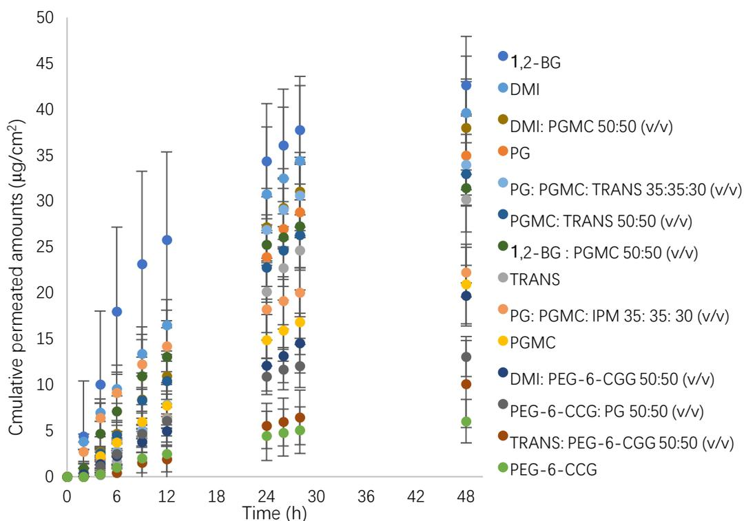
**Figure 6.13** Permeation profiles of caffeine from a range of different solvents and solvent mixtures in Franz cells with human skin. Each data point represents the mean  $\pm$  SD, n=5.
