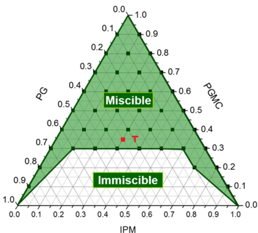
**Figure 6.9** Ternary phase diagram of PG: PGMC: IPM system [T-PG: PGMC: IPM (35:35:30 v/v)]. The original ternary phase diagram with other selected compositions was constructed by Hadi (2012).
