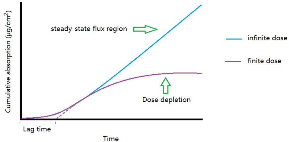
**Figure 3.2** Typical permeation profiles for an infinite dose and a finite dose study
