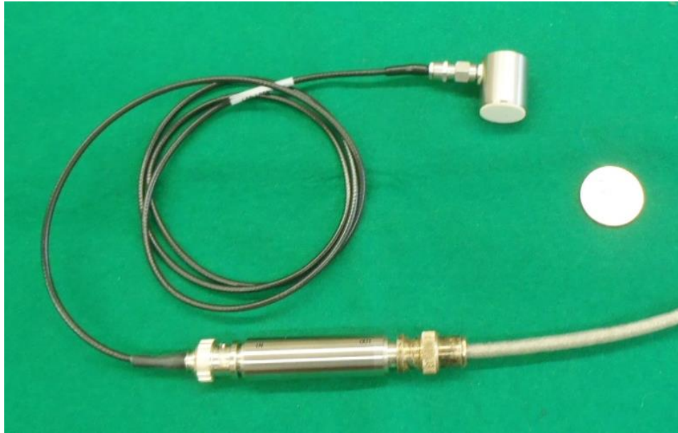
Figure 3. Typical AE sensor and pre-amplifier for a laboratory experiment. Coin is 24.26 mm in diameter (a quarter of US dollar) for scale.
